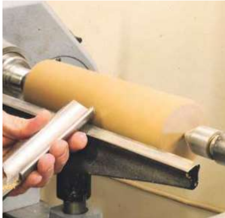
▲ Pic.2 Mount the oak between centres and make it round using the centre – the strongest part – of the spindle roughing gouge. The wings of the tool can be used for the fine finishing cuts
